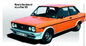
are still less than £12k. Built from 1978 to 1984 they had wheelarch extensions, bib spoiler, cheese-cutter grille, short-throw gearshift, alloys and air horns. The 114bhp 2.0-litre twin cam wasn't that quick at 110mph – but find one in bright orange and I guarantee you'll be properly captivated.
